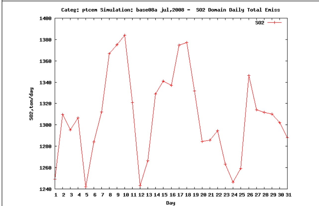
Figure 6. Daily variation in CEM Point Source NO x (top) and SO 2 (bottom) emissions across the 4 km Inter-Mountain West Modeling Domain for July 2008.
